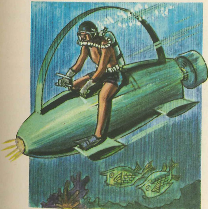
A battery-driven diving vehicle with a scuba diver astride.
